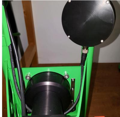
Fit WiFi cable to the transmitter and clip to the frame as shown above. Route the cable under the hub and upwards towards the Display Unit
