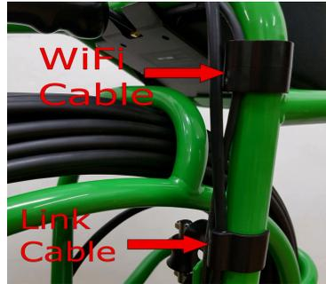
Fit the end of the cable to the EXT VIDEO socket on the Display Unit and clip the cable as shown above - ensure there are no tight bends of the cable as the Display Unit is put in the upright position.
