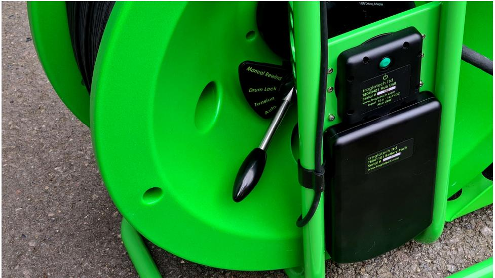
The only external difference between the manual and auto drums is the addition of the control lever as seen above. But hidden in the centre of the hub is a three-phase brushless motor and Troglotech-designed Cycloid gearbox providing enough power to retrieve 300m of cable and the crawler at 0.5M/S
